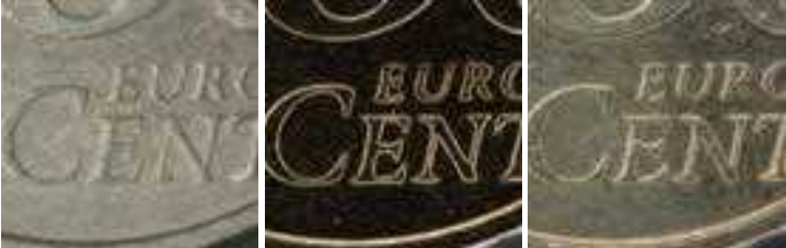
Reflected light, brightfield, quarter circle Reflected light darkfield, full circle Mixed light, combination of brightfield and darkfield While darkfield illumination brings out the raised contours of this 50-cent coin, mixed-light illumination reveals irregularities on the surface.
