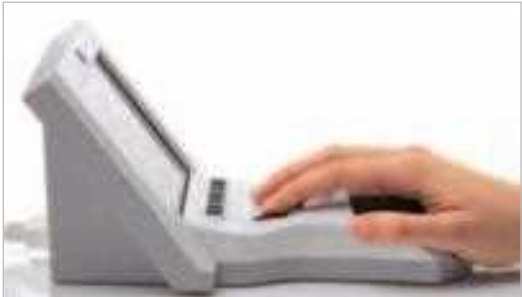
The two scroll wheels are used for fine focus adjustments. A click is all it takes to switch to the fine X-axis and Y-axis controls for the motorized stage.
