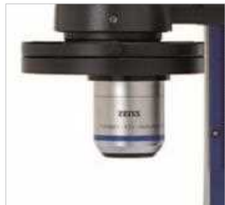
Objective PlanApo S 3.5x mono on Objective slider S/doc ■ For axial mode only ■ Free working distance FWD = 16 mm ■ Max. possible resolution of 1,510 LP/mm (equals 0.3 \mu m)
