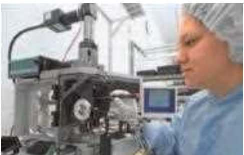
The precise movement of all the moving optical elements in the optical train is programmed on the zoom lens system adjustment device. Around 7,000 support points are analyzed in a computer for this purpose. This ensures that each individual stereo microscope gets its own fine-tuning calibration and its own individual zoom curve.
