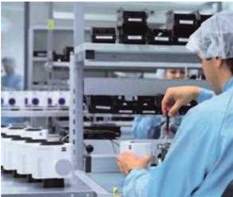
Fast, flexible, effective: SteREO Discovery stereo microscopes undergoing final assembly at the Carl Zeiss Microscopy GmbH clean rooms in Jena. The method? One-piece continuous flow manufacturing based on value stream design criteria.
