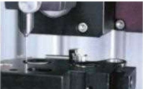
Once the lens has been pushed into position, it is fixed in place immediately. A 0.5 mm thick cannula is used by high-precision tools to automatically apply continuous adhesive beads with high accuracy and precision.
