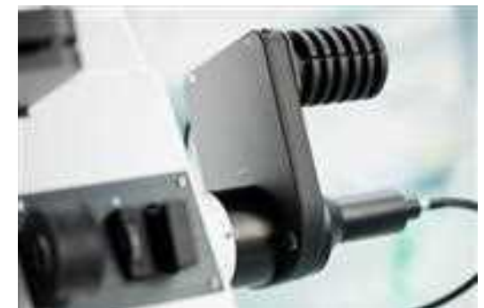
Excitation filter wheel for high speed multicolor imaging.
