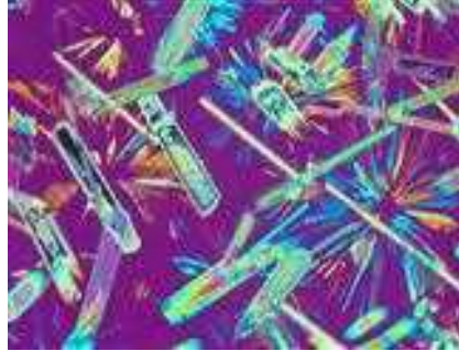
Crystal, acquired in polarization contrast, objective: Plan-Neofluar 20x/0.8
